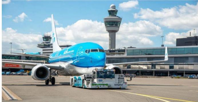
The motivation for this is significant reduction in fuel use and noise. Known as the *TaxiBot*, it is a semi-robotic hybrid towing vehicle made by **Smart Airport Systems** under license from **Israel Aircraft Industries** for taxiing airplanes with their power off. The company claims that its AV can reduce CO2 emissions by as much as 85%, noise pollution by 60%, and fuel by 65%. More information is at [this link](#).
