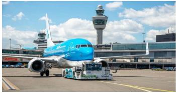
reduction in fuel use and noise. Known as the *TaxiBot*, it is a semi-robotic hybrid towing vehicle made by **Smart Airport Systems** under license from **Israel Aircraft Industries** for taxiing airplanes with their power off. The company claims that its AV can reduce CO2 emissions by as much as 85%, noise pollution by 60%, and fuel by 65%. More information is at this link.
